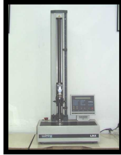
Resim 3. Universal test cihazı (Lloyd-LRX Universal/Fareham, England).
