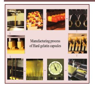
Figure 5: Manufacturing process of hard gelatin capsule[5].
