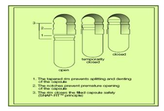
Figure 7: Recent hard gelatin capsule with features (notches or dimples) for pre-closing; closing features (e.g. SNAP-FIT<sup>™</sup>) and tapered rim (e.g. CONI-SNAP<sup>™</sup>).
