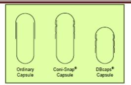
Figure 8: Drawings of an ordinary capsule (left), a Coni-Snap<sup>®</sup> capsule (center) and a DBcaps<sup>®</sup> capsule (right). In Coni-Snap<sup>®</sup> and DBcaps<sup>®</sup> capsules, the tapered rim of the body is designed to avoid telescoping, the grooves on cap and body lock together; the presence of indentations prevents premature opening.
