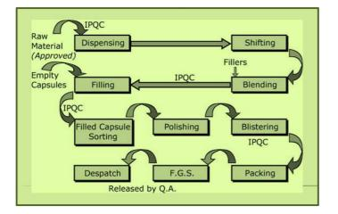
Figure 1: Flow chart for Capsule manufacturing steps.
