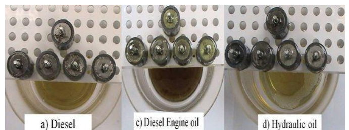
Figure 3. Sorbent fibrous assemblies for static sorption using the three sorbates.
