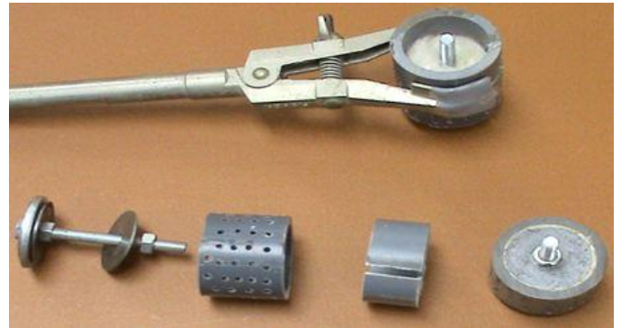
Figure 2. Construction manner of the fibrous assembly used for oil sorption.
