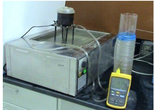
Figure 4. Static sorption of the three oil sorbents by the fibrous assemblies under controlled temperature
