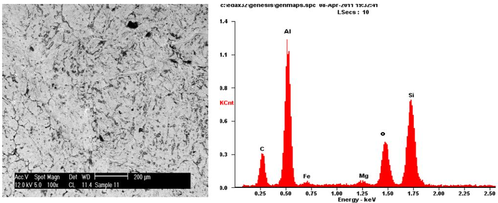
**Fig. 5** SEM/EDS of the aluminium alloy reinforced with 20 wt% rice husk ash
