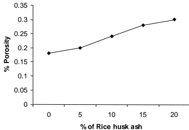
**Fig. 7** Variation of percentage of porosity with weight percentage of rice husk ash addition
