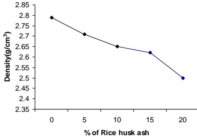
**Fig. 6** Variation of density with weight percentage of rice husk ash addition
