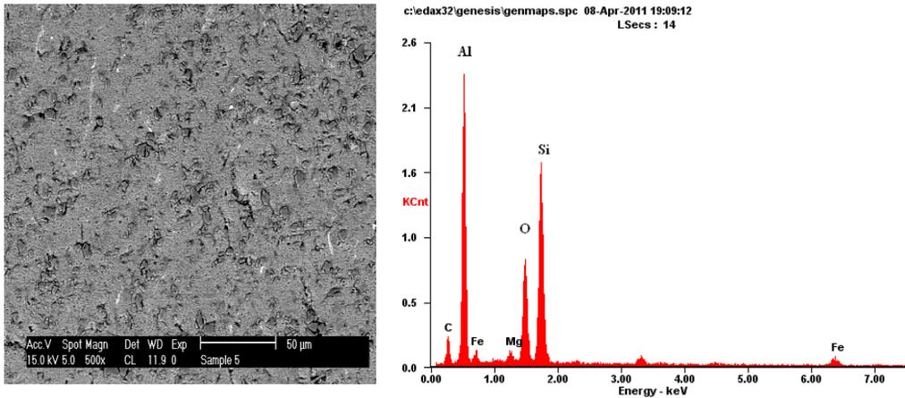
**Fig. 4** SEM/EDS of the aluminium alloy reinforced with 10 wt% rice husk ash
