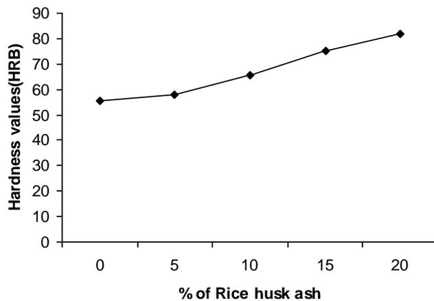
**Fig. 10** Variation of hardness values with weight percentage of rice husk ash addition
