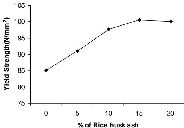
**Fig. 8** Variation of Yield Strength with weight percentage of rice husk ash addition
