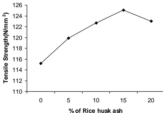
**Fig. 9** Variation of Tensile Strength with weight percentage of rice husk ash addition
