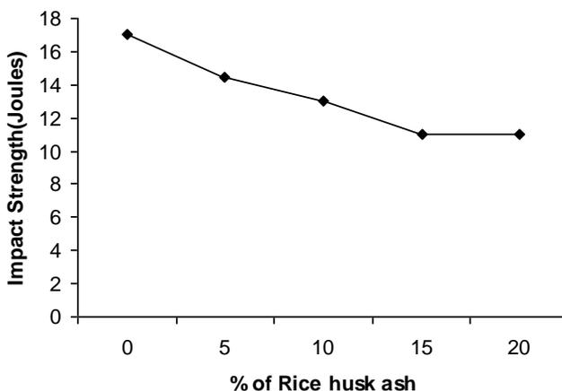
**Fig. 11** Variation of Impact energy with weight percentage of rice husk ash addition
