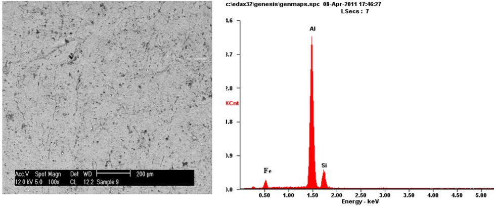
**Fig. 3** SEM/EDS of the aluminium alloy
