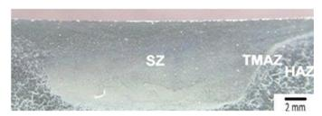
Fig. 2 Macrostructure of Different Regions of FSW joints
