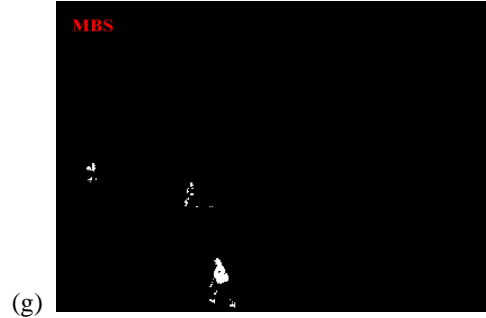
Fig. 4 Detected results on a frame that contains obvious sunshine change: (a) original frame- frame 2383, (b) the result of ABS, (c) the result of MOG, (d) the result of NPK, (e) the second layer of Gauss pyramid, (f) detected result on the low-resolution level , (g) the result of MBS(our method)
