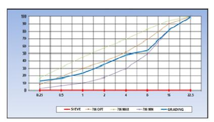
Figure 5. Granulometry curve for proposed mixture
