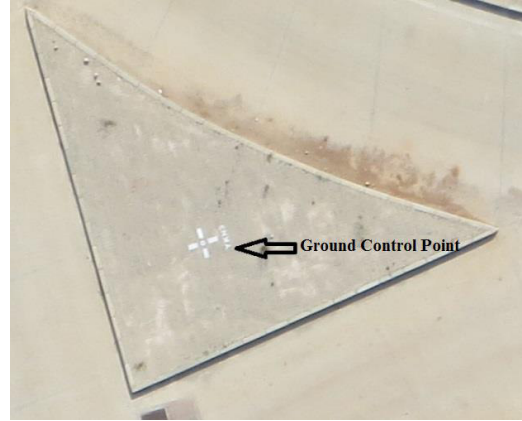
Figure 5. Ground control point established on the land for orthomosaic
