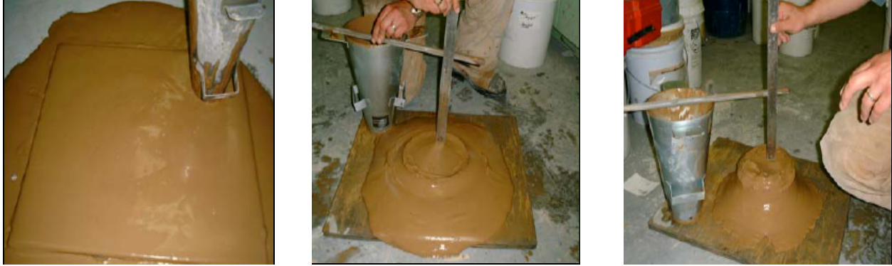
Figure 2. Slumps; Slurry (a), 250 mm Slump Paste (b), 175 mm Slump Paste (c) (Grabinsky et al., 2002).
