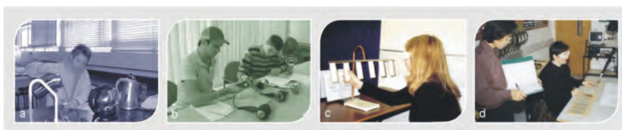
a, b - sensory evaluation tests within product context (kettles and hair dryers) c, d - sensory tests of isolated material samples (elastomer and metals)
