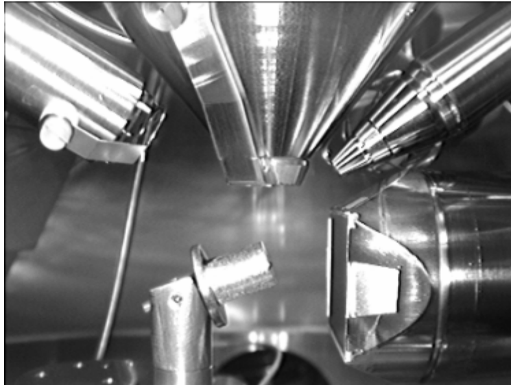
Figure 6. A sample processed by 8 passes of ECAP is located in EBSD test chamber.
