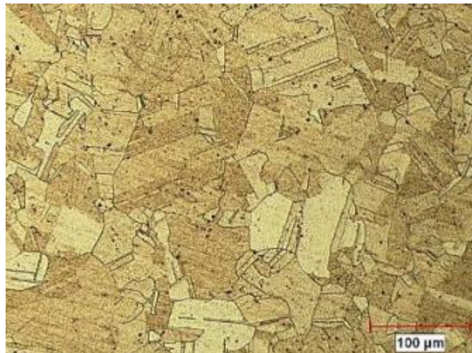
Figure 7. The unECAPed sample with a grain size of 60.8 micrometer.
