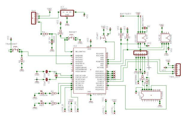
Figure 3. Control and recording circuit
