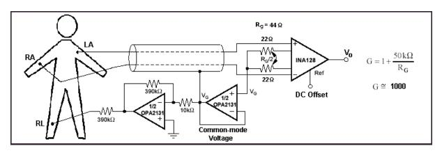
Figure 1. Instrumentation amplifier circuit
