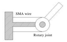
Fig.1 Two wire rotary actuators configuration
