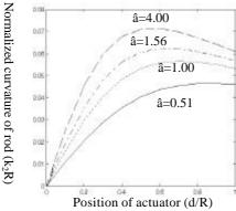
Fig.4 Maximum deflection of the rod versus the normalized position of the actuator
