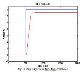
The step response, although smooth, never reaches the set point, and has a steady state error of 1.15. The rise time, measured from the 10% to the 90% of the final value is, 105 ms with a 85 ms delay.
