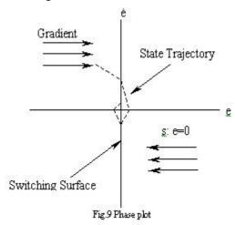
With properly chosen feedback gains, the state trajectory can be constrained to move along the switching surface after the initial intersection with the switching surface. Such a motion along a switching surface is referred to as a "sliding mode", and exists on a discontinuity surface whenever the distance to this surface and the velocity of its change are of opposite signs [10]. More specifically:
