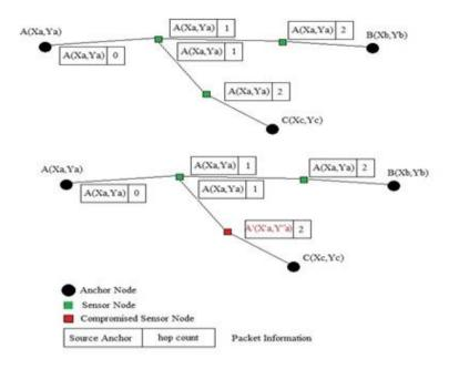
FIGURE 2. Node Compromise attack by the attacker sensor node with the manipulation of the anchor node's location
