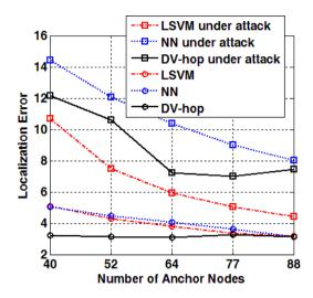
FIGURE 6. The effect of different number of the compromised anchor node compromise attack on the localization algorithms
