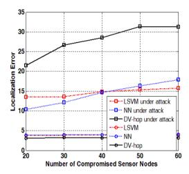
FIGURE 7. The effect of different number of the compromised sensor nodes & sensor node compromise attack on localization accuracy
