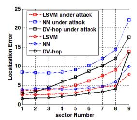
FIGURE 13. Border problem in case of attack and no attack in three runs with 64 anchors
