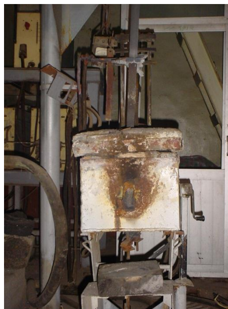
Figure 1. Photograph of the Baby Electric Arc Furnace used for preliminary fusion tests
