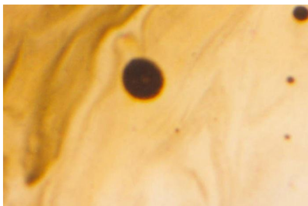
Figure 3. Photomicrograph of fused silica product from Electric Arc Furnace showing flowage texture staining with iron oxide. Plain polarized light
