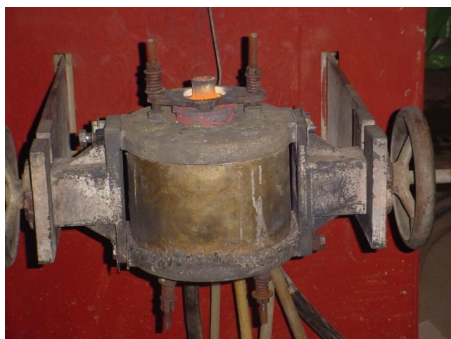
Figure 2. The Tamman Furnace used in production of fused silica
