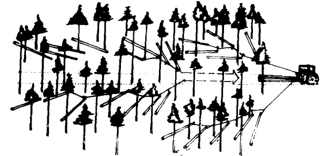
Şekil : 2 — Vinçle mücehhez traktörle dağlık arazide nakliyat Fig : 2 — Skidding with tractor mounted winches in mountainous regions
