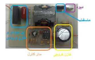
Figure 8. Sample of Boost PFC converter.
