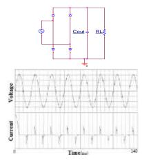
Figure 1. Voltage rectifier along with input voltage and current waveforms.
