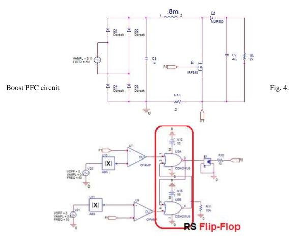
Figure 5. Boost PFC converter control circuit.
