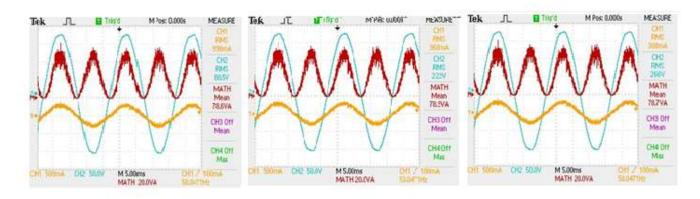
Figure 9. Voltage, current, and input power wave forms.
