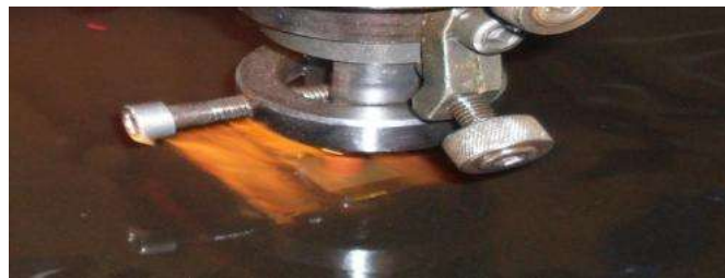
Figure 8. Workpiece and the tool installed and ready for machining
