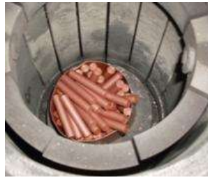
Figure 3. Due to the use of vacuum furnace, the specimen surface was not oxidized with any impurity.
