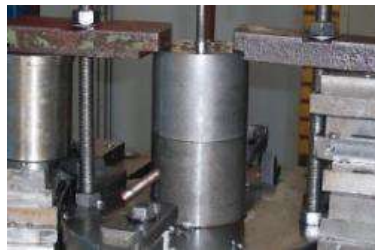
Figure 4. The copper specimen is removed from the ECAP die
