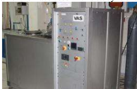
Figure 2. The VAS furnace is made in France and, with its graphite elements, allows for heat treatment under vacuum up to 10^{-2} Torr and up to 1500 °C. It has a controlled and programmable heating cycle.
