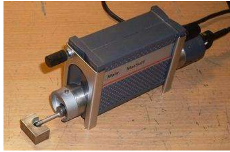
Figure 9. Surface roughness measurement using the Mahr device
