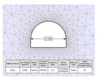
Figure 2. Numerical modeling of the tunnel No.2 of Kurdistan
