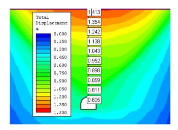
Figure 3. Displacements in the tunnel roof in deterministic analysis
