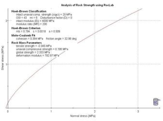
Figure 1. The geomechanical parameters of shale rock masses
