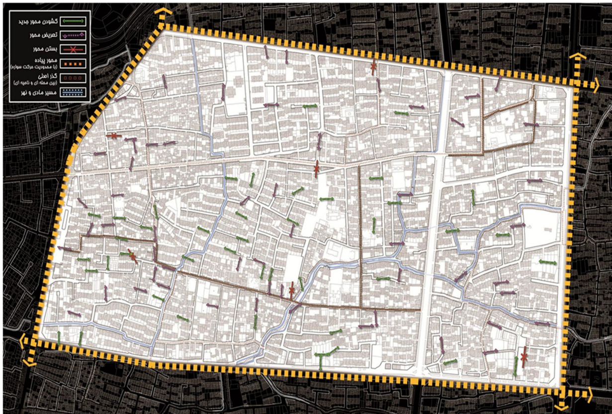
Fig. 10. Alternative no.2 for the design: Proposed modifications in the axes within the area and Selection of Pedestrian-based Route
