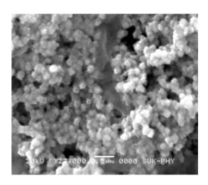
Figure.3. Reduction of Ag<sup>+</sup> ions Fig.4 SEM Micrograph of silver nanoparticles:
