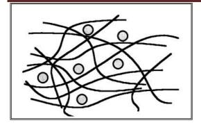
FIG. 4 Amorphous solid solution
