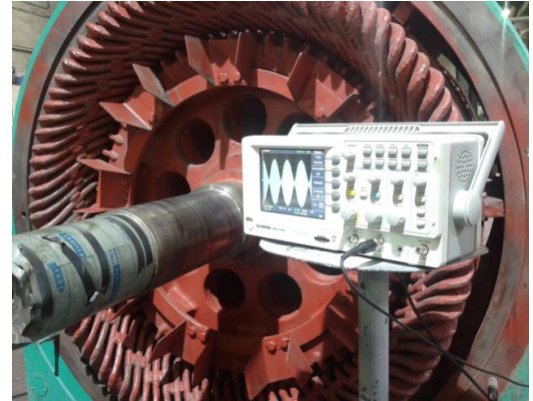
Fig.6. Schematic machine with the coil under test
