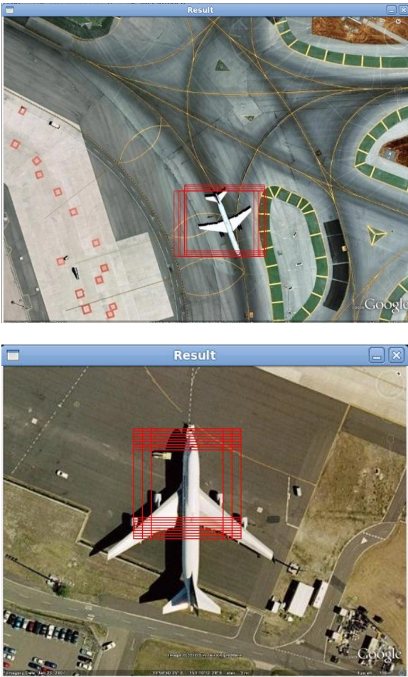
Figure 7 (cont.). Aircraft detection results. Red boxes show the detected aircrafts in that region.
