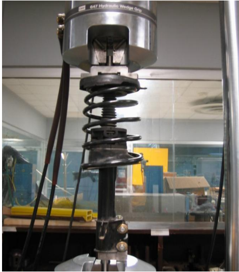
Fig. 7 Obtaining data from spring and damper in a Universal machine
