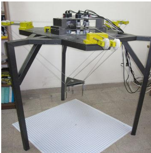
Fig. 13 Scheme of the designed IUST cable robot [15]
