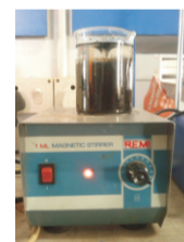
Figure 1: Preparation of Mg-Np's using Magnetic stirrer
