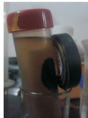
Figure 3: Chitosan coated Mg-Np's with bacterial solution for magnetic separation
