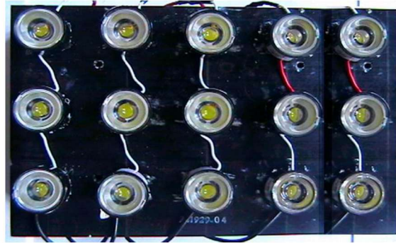
Figure 4. The LED array on the PCB (5 parallel columns of 3 series LEDs on an aluminum PCB, the LED driver is at the back of the PCB)
