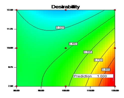
Figure 4. Contour plot showing relationship between various levels of HPMC and NaHCO3 to attain fixed value of floating lag time.
