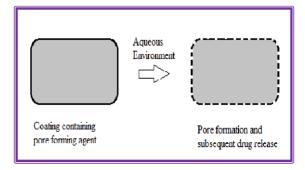
Figure 8: Controlled porosity osmotic pump
