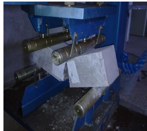
Figure 7. Flexural strength test
