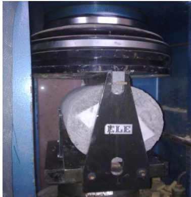
Figure 9. Indirect tensile strength test
