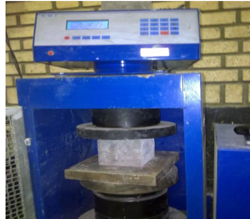
Figure 3. Compressive strength test
