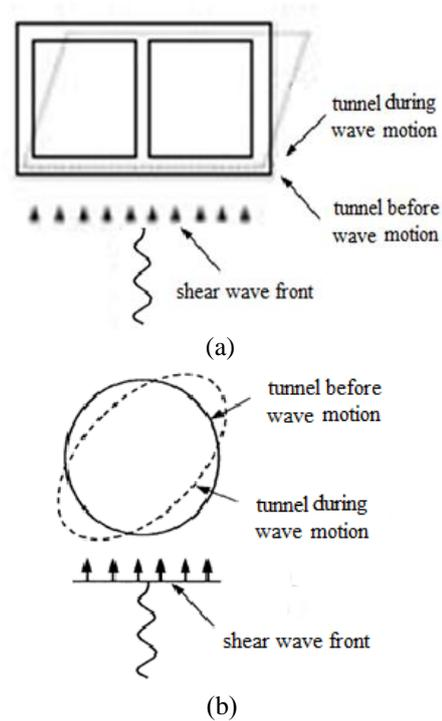
Figure 2. (a) Racking Deformation of a Rectangular Cross Section (b) Ovaling Deformation of a Circular Cross Section
