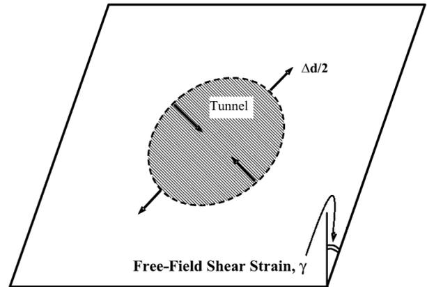
Figure 5. Free-field shear distortion of perforated (tunnel cavity is empty) and non-perforated ground (tunnel cavity is filled), circular shape
