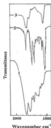
Figure 166. FT-IR spectra of BSA (1), betulin (2), and the products obtained from the BSA + betulin + carbodiimide mixture (3).
