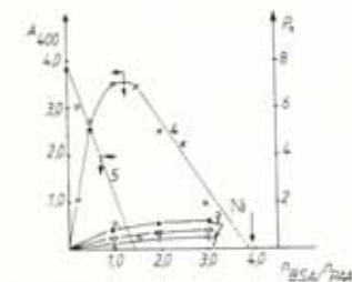
Figure 81. Turbidimetric titration of PAA- Cu^{2+} mixture with the solution of BSA. (1-4) Dependence of optical density ( A_{400} ) of ternary mixture PAA- Cu^{2+} -BSA on n_{BSA}/n_{PAA} at difference n_{Cu}/n_{AA} : 0.08(1); 0.1 (2); 0.2 (3); 0.3 (4). (5) Dependence of the area of the free PMC peaks ( P_0 ) on the ratio n_{ESANFAA} obtained in matrix solution of ternary mixture at n_{Cu}/n_{AA} = 0.3\ C_{PAA} = 0.1\ g/dL; pH\ 7; 25^\circ C .
