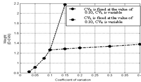
**Figure 6.** Graphical representation of the coefficient of variation versus the weight of the bridge
