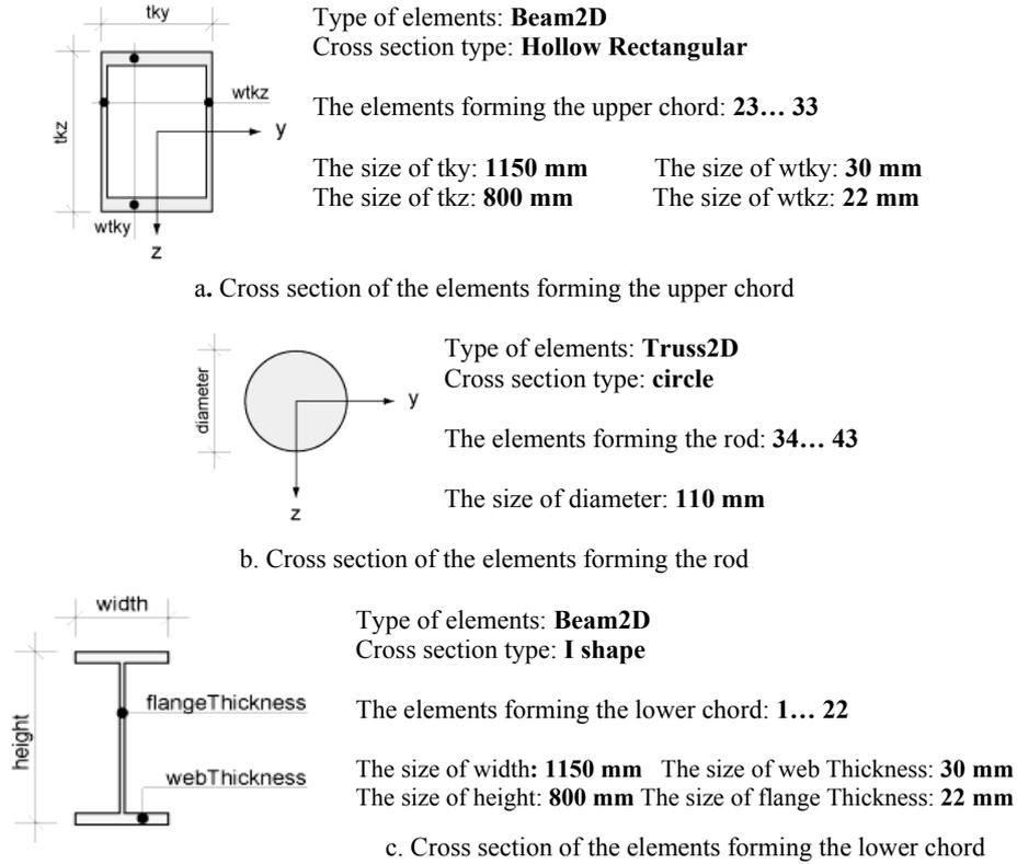
**Figure 4.** Properties of the cross sections used in the steel arch bridge
