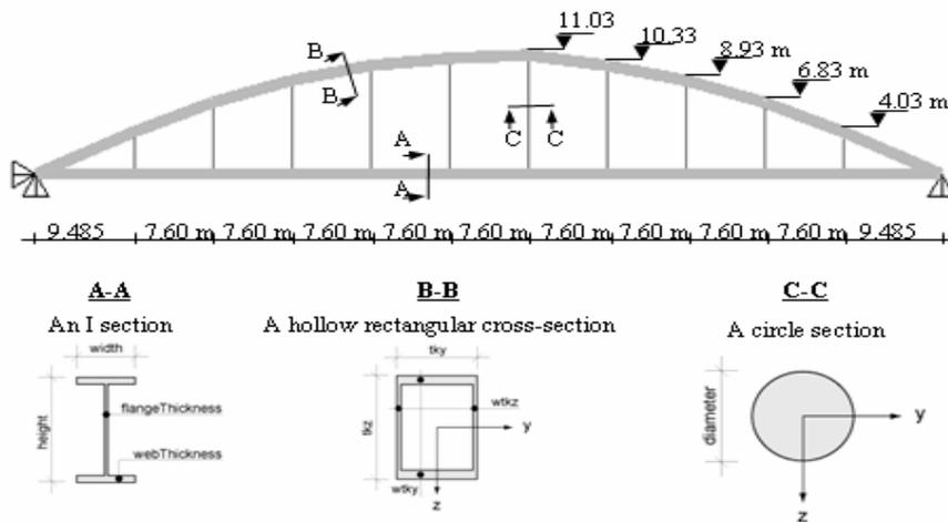
Figure 2. The topology and geometrical properties of the cross-section of 2D Arch Bridge
