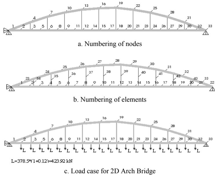
Figure 3. The definition of 2D Arch Bridge
